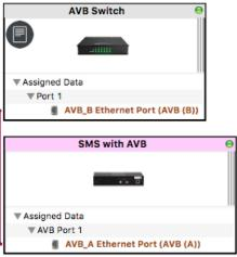
The Savant IP Audio devices Ethernet port must be connected to the AVB switch.
